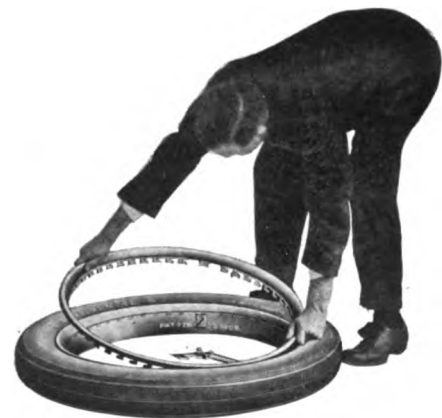
Fig. 5—Putting the outer rim in place
